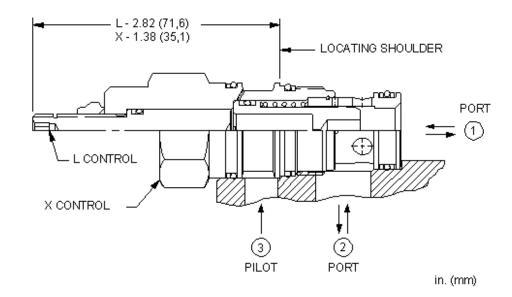
These unbalanced, pilot-to-close logic valves are 2-way switching elements that are spring biased open. Pressure at either work port 1 or 2 will tend to keep the valve open while pressure at port 3 will tend to close it. The force generated at port 3 must be greater than the sum of the forces acting at port 1 and port 2 plus the spring force for the valve to close. NOTE: The pilot area (port 3) is 1.8 times the area at port 1 and 2.25 times the area at port 2.
