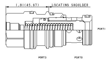
This valve is an unbalanced, vent-to-open, 2-way logic switching element with an integral pilot control cavity. It is spring biased closed and uses port 2 as a pilot source. With a pilot 2-way valve in the closed position installed in the T-8A
