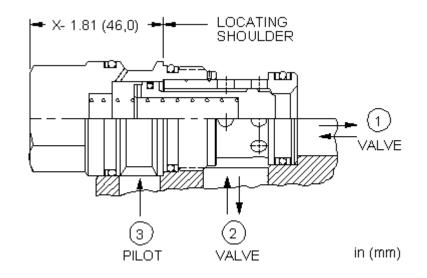
These unbalanced, pilot-to-close logic valves are 2-way switching elements that are spring biased closed. Pressure at either work port 1 or 2 will oppose the spring and tend to open the valve while pressure at port 3 will tend to close it. The force generated at port 3, plus the spring force, must be greater than the sum of the forces acting at port 1 and port 2 for the valve to remain closed. NOTE: The pilot area (port 3) is 1.8 times the area at port 1 and 2.25 times the area at port 2.
