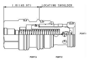
This valve is an unbalanced, vent-to-open 2-way logic switching element with an integral pilot control cavity. It is
