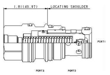
This valve is an unbalanced, vent-to-open 2-way logic switching element with an integral pilot control cavity. It is spring biased closed and incorporates an integral shuttle so
