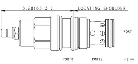
These unbalanced, pilot-to-close logic valves are 2-way switching elements that are spring biased closed. Pressure at either work port 1 or 2 will oppose the spring and tend to open the valve while pressure at port 3 will tend to close it. The force generated at port 3, plus the spring force, must be greater than the sum of the forces acting at port 1 and port 2 for the valve to remain closed. NOTE: The pilot area (port 3) is 1.8 times the area at port 1 and 2.25 times the area at port 2.
