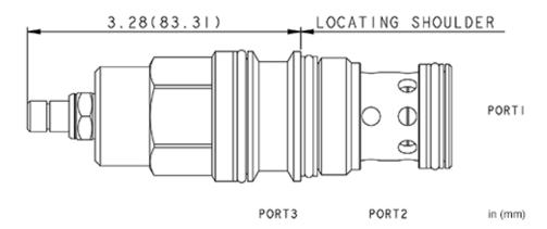
These unbalanced, pilot-to-close logic valves are 2-way switching elements that are spring biased closed. Pressure at either work port 1 or 2 will oppose the spring and tend to open the valve while pressure at port 3 will tend to close it. The force generated at port 3, plus the spring force, must be greater than the sum of the forces acting at port 1 and port 2 for the valve to remain closed. NOTE: The pilot area (port 3) is 1.8 times the area at port 1 and 2.25 times the area at port 2.
