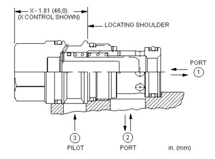
These unbalanced, pilot-to-close logic valves are 2-way switching elements that are spring biased open. Pressure at either work port 1 or 2 will tend to keep the valve open while pressure at port 3 will tend to close it. The force generated at port 3 must be greater than the sum of the forces acting at port 1 and port 2 plus the spring force for the valve to close. NOTE: The pilot area (port 3) is 1.8 times the area at port 1 and 2.25 times the area at port 2.
