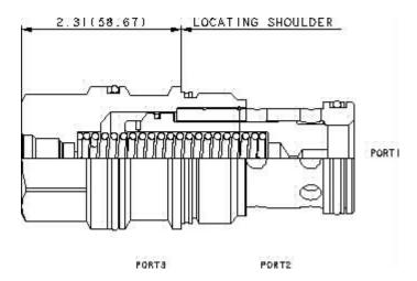
This valve is an unbalanced, vent-to-open, 2-way logic switching element with an integral pilot control cavity. It is spring biased closed and uses port 1 as a pilot source. With
