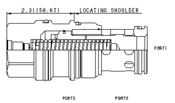
This valve is an unbalanced, vent-to-open, 2-way logic switching element with an integral pilot control cavity. It is spring biased closed and uses port 2 as a pilot source. With a pilot 2-way valve in the closed position installed in the T-8A
