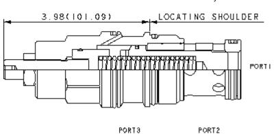
These unbalanced, pilot-to-close logic valves are 2-way switching elements that are spring biased closed. Pressure at either work port 1 or 2 will oppose the spring and tend to open the valve while pressure at port 3 will tend to close it. The force generated at port 3, plus the spring force, must be greater than the sum of the forces acting at port 1 and port 2 for the valve to remain closed. NOTE: The pilot area (port 3) is 1.8 times the area at port 1 and 2.25 times the area at port 2.
