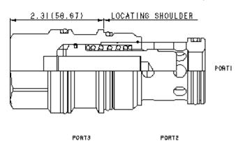
These unbalanced, pilot-to-close logic valves are 2-way
