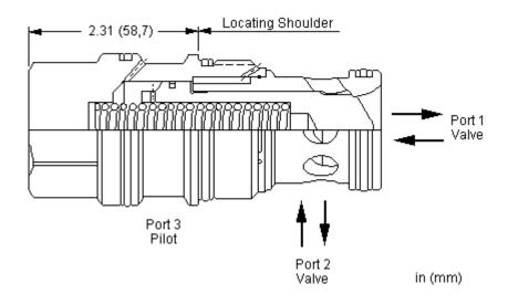
These unbalanced, pilot-to-close logic valves are 2-way switching elements that are spring biased closed. Pressure at either work port 1 or 2 will oppose the spring and tend to open the valve while pressure at port 3 will tend to close it. The force generated at port 3, plus the spring force, must be greater than the sum of the forces acting at port 1 and port 2 for the valve to remain closed. NOTE: The pilot area (port 3) is 1.8 times the area at port 1 and 2.25 times the area at port 2.
