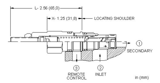
These normally open modulating elements with an internal orifice between port 1 and port 3 can be used as a main-stage reducing valve. The valve can be controlled remotely using a pilot relief or pilot solenoid valve.
