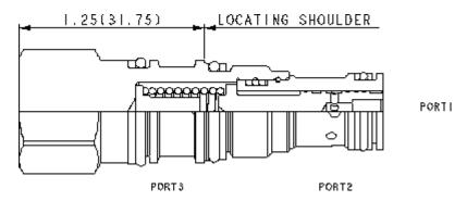
This normally open modulating element is specifically designed to work with our accumulator sense, pump unload pilot valve to provide a soft unload.
