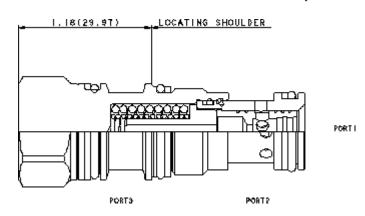
These normally open modulating elements with an internal orifice between port 1 and port 3 can be used as a main-stage reducing valve. The valve can be controlled remotely using a pilot relief or pilot solenoid valve.
