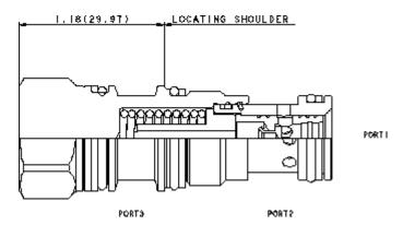
Normally open modulating elements without an internal orifice act as a restrictive compensator to maintain a constant pressure drop across an orifice, regardless of variations in upstream or downstream pressure.
