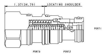
Normally open modulating elements without an internal orifice act as a restrictive compensator to maintain a constant pressure drop across an orifice, regardless of variations in upstream or downstream pressure.
