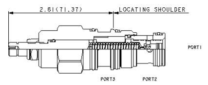
Normally open modulating elements without an internal orifice act as a restrictive compensator to maintain a constant pressure drop across an orifice, regardless of variations in upstream or downstream pressure.
