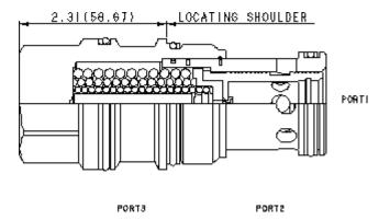
These normally open modulating elements with an internal orifice between port 1 and port 3 can be used as a main-stage reducing valve. The valve can be controlled remotely using a pilot relief or pilot solenoid valve.
