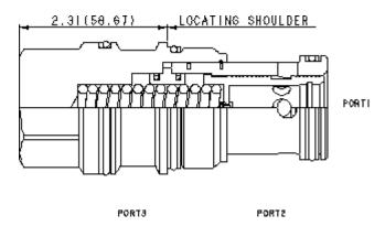
Normally open modulating elements without an internal orifice act as a restrictive compensator to maintain a constant pressure drop across an orifice, regardless of variations in upstream or downstream pressure.
