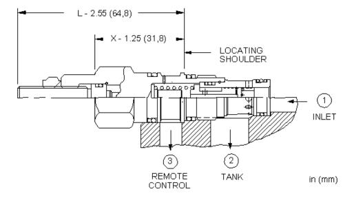
Normally closed modulating elements with an internal orifice between port 1 and port 3 can be used as a mainstage relief valve. The valve can be controlled remotely using a pilot relief or pilot solenoid valve.
