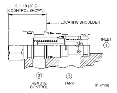
Normally closed modulating elements with an internal orifice between port 1 and port 3 can be used as a mainstage relief valve. The valve can be controlled remotely using a pilot relief or pilot solenoid valve.
