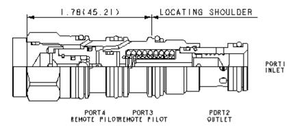
A normally closed modulating element, used as a bypass compensator, ensures a constant pressure drop across an external orifice to create a pressure compensated flow control. The resulting flow remains constant regardless of variations in upstream or downstream pressure. A ball shuttle connects the after orifice signal from the higher of port 3 or 4 to the pilot area.
