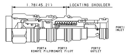
A normally closed modulating element, used as a bypass compensator, ensures a constant pressure drop across an external orifice to create a pressure compensated flow control. The resulting flow remains constant regardless of variations in upstream or downstream pressure. A ball shuttle connects the after orifice signal from the higher of port 3 or 4 to the pilot area.
