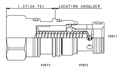
Normally closed modulating elements without an internal orifice act as a bypass compensator to maintain a constant pressure drop across an orifice, regardless of variations in upstream or downstream pressure.
