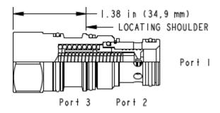
Normally closed modulating elements without an internal orifice act as a bypass compensator to maintain a constant pressure drop across an orifice, regardless of variations in upstream or downstream pressure.
