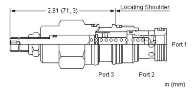
Normally closed modulating elements without an internal orifice act as a bypass compensator to maintain a constant pressure drop across an orifice, regardless of variations in upstream or downstream pressure.
