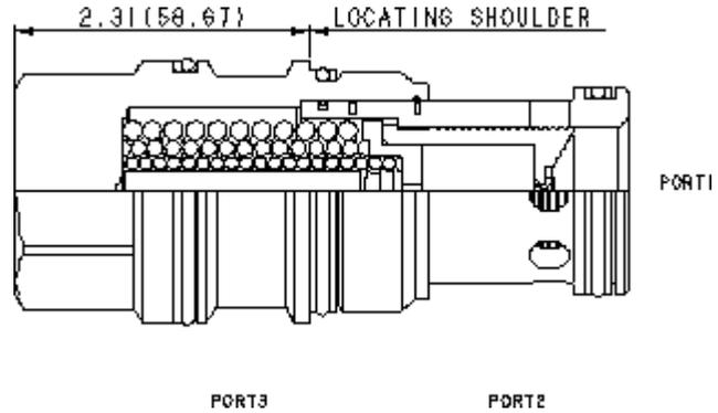
Normally closed modulating elements with an internal orifice between port 1 and port 3 can be used as a main-stage relief valve. The valve can be controlled remotely using a pilot relief or pilot solenoid valve.
