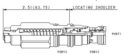
Load reactive, load control valves with pilot assist combine two valves; a check valve and a relief valve. The check valve allows free flow from the directional valve (port 2) to the load (port 1) while a direct-acting, pilot-assisted relief valve controls flow from port 1 to port 2. Pilot assist at port 3 lowers the effective setting of the relief valve at a rate determined by the pilot ratio.
