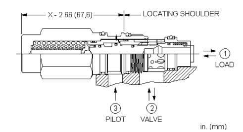
Fixed setting, load reactive, load control valves with pilot assist combine two valves; a check valve and a relief valve. The check valve allows free flow from the directional valve (port 2) to the load (port 1) while a direct-acting, pilot-assisted relief valve controls flow from port 1 to port 2. Pilot assist at port 3 lowers the effective setting of the relief valve at a rate determined by the pilot ratio.
