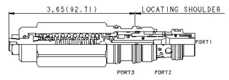
Load reactive, load control valves with pilot assist combine two valves; a check valve and a relief valve. The check valve allows free flow from the directional valve (port 2) to the load (port 1) while a direct-acting, pilot-assisted relief valve controls flow from port 1 to port 2. Pilot assist at port 3 lowers the effective setting of the relief valve at a rate determined by the pilot ratio.
