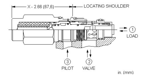
Fixed setting, load reactive, load control valves with pilot assist combine two valves; a check valve and a relief valve. The check valve allows free flow from the directional valve (port 2) to the load (port 1) while a direct-acting, pilot-assisted relief valve controls flow from port 1 to port 2. Pilot assist at port 3 lowers the effective setting of the relief valve at a rate determined by the pilot ratio.
