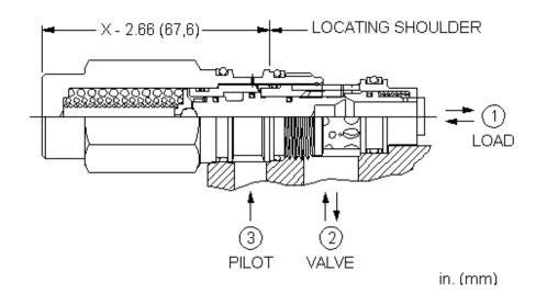
Balanced load control valves combine a balanced modulating element with a reverse flow check. The check valve allows free flow from the directional valve (port 2) to the load (port 1) while the pilot to open modulating element controls flow from port 1 to port 2. Pilot pressure at port 3 determines the flow setting.
