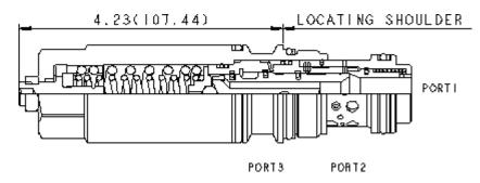
Load reactive, load control valves with pilot assist combine two valves; a check valve and a relief valve. The check valve allows free flow from the directional valve (port 2) to the load (port 1) while a direct-acting, pilot-assisted relief valve controls flow from port 1 to port 2. Pilot assist at port 3 lowers the effective setting of the relief valve at a rate determined by the pilot ratio.
