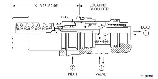
Fixed setting, load reactive, load control valves with pilot assist combine two valves; a check valve and a relief valve. The check valve allows free flow from the directional valve (port 2) to the load (port 1) while a direct-acting, pilot-assisted relief valve controls flow from port 1 to port 2. Pilot assist at port 3 lowers the effective setting of the relief valve at a rate determined by the pilot ratio.
