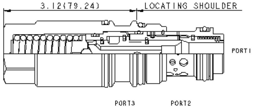
Balanced load control valves combine a balanced modulating element with a reverse flow check. The check valve allows free flow from the directional valve (port 2) to the load (port 1) while the pilot to open modulating element controls flow from port 1 to port 2. Pilot pressure at port 3 determines the flow setting.
