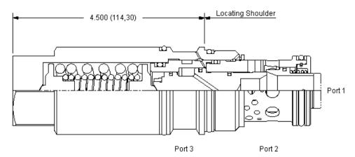
Fixed setting, load reactive, load control valves with pilot assist combine two valves; a check valve and a relief valve. The check valve allows free flow from the directional valve (port 2) to the load (port 1) while a direct-acting, pilot-assisted relief valve controls flow from port 1 to port 2. Pilot assist at port 3 lowers the effective setting of the relief valve at a rate determined by the pilot ratio.
