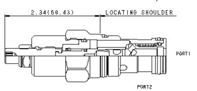
Needle valves with reverse-flow check are fully adjustable orifices used to regulate flow. They are infinitely adjustable from fully closed up to the maximum orifice diameter. An integral high-capacity check valve provides unrestricted flow from port 2 to port 1. They are not pressure compensated.
