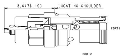
Needle valves with reverse-flow check are fully adjustable orifices used to regulate flow. They are infinitely adjustable from fully closed up to the maximum orifice diameter. An integral high-capacity check valve provides unrestricted flow from port 2 to port 1. They are not pressure compensated.
