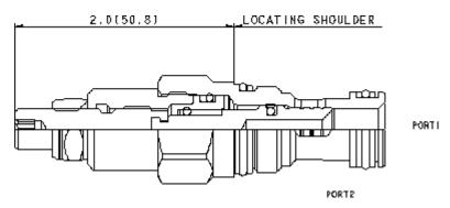
Needle valves are fully adjustable orifices used to regulate flow. They are infinitely adjustable from fully closed up to the maximum orifice diameter. They are not pressure compensated and may be used as flow controls or as shutoff valves.
