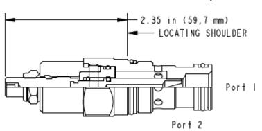
Needle valves are fully adjustable orifices used to regulate flow. They are infinitely adjustable from fully closed up to the maximum orifice diameter. They are not pressure compensated and may be used as flow controls or as shutoff valves.
