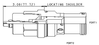
Needle valves are fully adjustable orifices used to regulate flow. They are infinitely adjustable from fully closed up to the maximum orifice diameter. They are not pressure compensated and may be used as flow controls or as shutoff valves.
