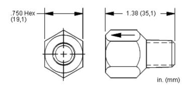
SUN gage line fuses protect systems from loss of oil if a gage or signal line breaks. If an object hits the gage or the fuse and breaks off the hex of the fuse, the line fuse will continue to perform its function because the working parts are located inside the port. The flow required to actuate the gage line fuse is 1.0 gpm (4 L/min).
