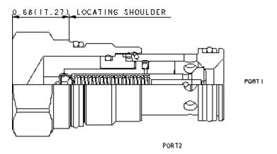
Air-bleed and start-up cartridges are used to purge air trapped in the system to help reduce power requirements and facilitate pump priming during the start-up of blocked center circuits.
