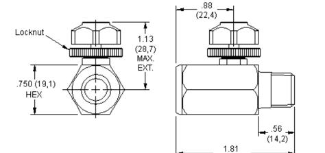
SUN adjustable gage snubbers are throttling and shut-off devices used to isolate and protect hydraulic gages from line pressure transients and the resulting gage pointer pulsations.
