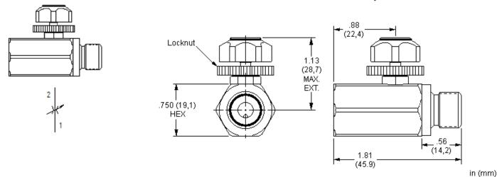
SUN adjustable gage snubbers are throttling and shut-off devices used to isolate and protect hydraulic gages from line pressure transients and the resulting gage pointer pulsations.
