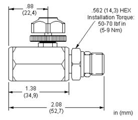
SUN adjustable gage snubbers are throttling and shut-off devices used to isolate and protect hydraulic gages from line pressure transients and the resulting gage pointer pulsations.
