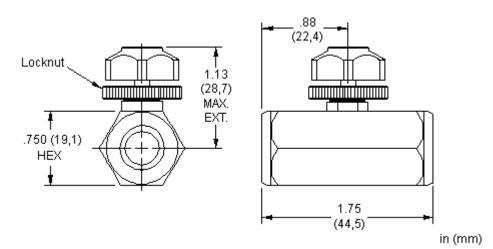
SUN adjustable gage snubbers are throttling and shut-off devices used to isolate and protect hydraulic gages from line pressure transients and the resulting gage pointer pulsations.
