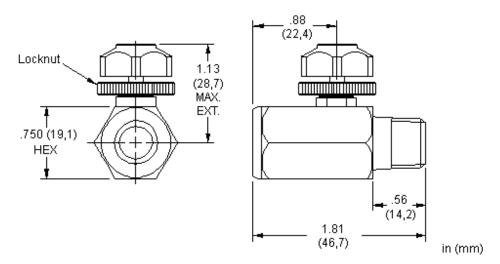
SUN adjustable gage snubbers are throttling and shut-off devices used to isolate and protect hydraulic gages from line pressure transients and the resulting gage pointer pulsations.
